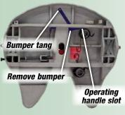
**Step 6:** Slide the bumper toward the operating handle slot and to the rear of the fifth wheel until the bumper tang clears the operating handle slot and remove.
