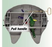
**Step 6:** Insert the pull handle through the fifth wheel skirt. Using the cotter pin and washer, fasten it to the top hole of the operating handle.
