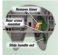
**Step 5:** Remove the timer by lifting upward. Then slide the operating handle out through the slot in the rear cross member of the fifth wheel.
