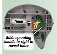
Step 4: Slide the operating handle over to the side of the fifth wheel. Slide the bottom part first. This will allow the underside of the handle to clear the jaw and wedge studs and timer.
