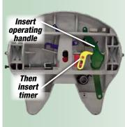
Step 4: Apply a liberal amount of grease to the grooved middle section of the operating handle. Insert the operating handle and move it over to the side of the wheel. Insert timer over the jaw and wedge studs. The small hole on the timer fits over the jaw stud and the slotted hole fits over the wedge stud. Be certain the small bent arm of the timer is facing downward.
