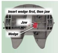
**Step 1:** Always assemble parts around a 2" kingpin or a shaft with a 2" diameter. Insert new jaw first and then the new wedge below it. Grease the jaw and wedge on top and bottom. Also apply grease to the stationary jaw in the throat of the fifth wheel.
