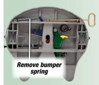
Step 1: Set the fifth wheel in a locked position (handle pushed in). Unhook the bumper spring from the bumper tang and the tab on the side of the fifth wheel substructure. Remove the bumper spring.
