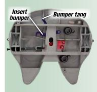
**Step 3:** Place the bumper back in position, sliding bumper tang through the operating handle guide slot and toward the tab on the side of the fifth wheel substructure.
