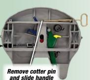
Step 2: Remove the cotter pin and washer that holds the pull handle to the operating handle. Slide the pull handle out through the side of the fifth wheel.
