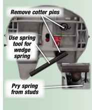
Step 7: CAUTION! The wedge spring is under extreme tension. Always wear safety glasses.
